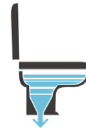
Washdown Flushing For Thorough Cleaning
